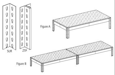
**3.** With the help from an associate, or using a wall for support, connect two SUR uprights (Ref. No. 1) using two front-to-back supports (Ref. No. 3), one at the top and one near the bottom (leaving the bottom-most keyhole slot empty). Be sure the front-to-back supports are fully seated in the keyhole slots as shown.
