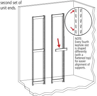
NOTE: If you are planning to install an adder unit, this second set of uprights should consist of ZTP uprights (Ref. No. 2) to act as an intermediate assembly. Carefully review step 2 to better understand.
