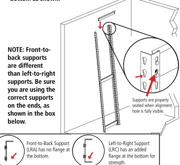
**4.** Place a third front-to-back support in the middle slots of the two uprights (at the level you want your third shelf to be). This forms one end of the shelving unit. Repeat steps 3 and 4 to construct a
