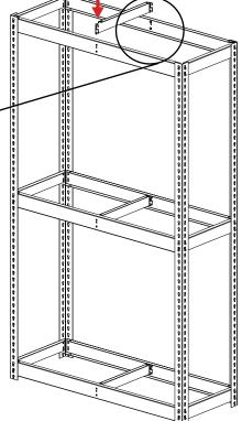
**8.** If particle board decking (Ref. No. 6) or wire decking (Ref. No. 7) was ordered, place the decking on each shelving level. The decking should fit flush inside the shelf supports. If you have purchased a single unit, your shelving unit is now complete. For adder units, see step 9.
