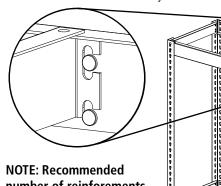
number of reinforements per shelf are as follows: 48"w = 1 reinforcement 60"w = 1 reinforcement 72"w = 2 reinforcement 96"w = 3 reinforcements
